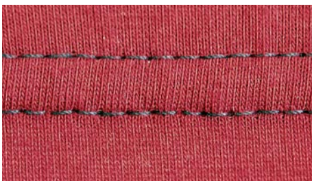
NO MORE MATERIAL DAMAGE VISIBLE – CORRECT NEEDLE THICKNESS HAS BEEN FOUND.
